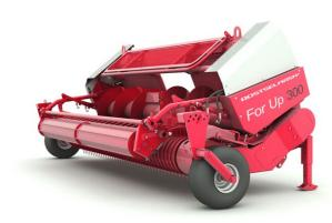
pickup (3 meter width) – provides collection of preliminary mowed and swathed grass.
