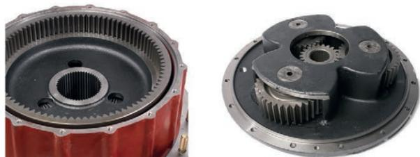
The planetary gears transfer all available power through the large precision helical gear. Planetary hubs are suspended on large bearings attached directly to the axle beam. The entire weight is supported by the axle beam, rather than the drive components
